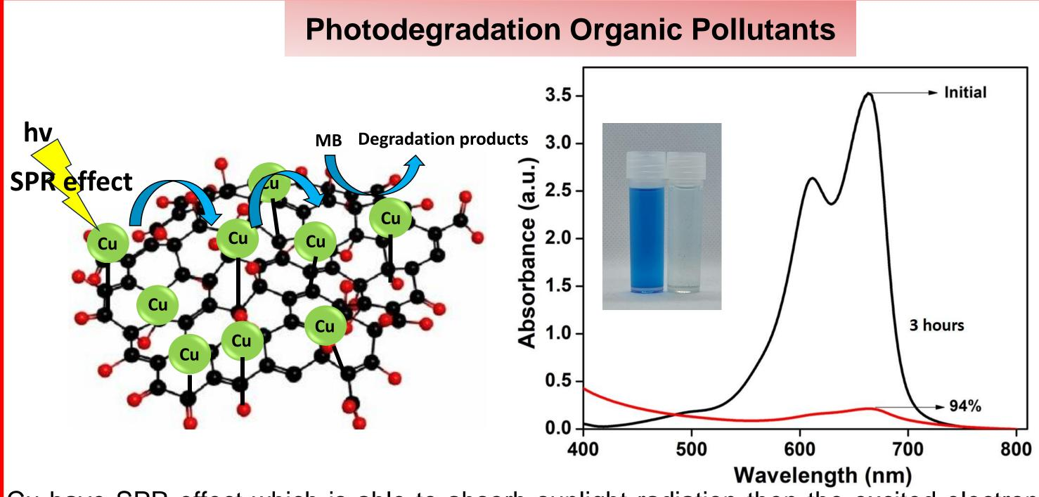
Cu have SPR effect which is able to absorb sunlight radiation then the excited electron transfer to GO via EDTA that electron react with the atmospheric oxygen to generate super oxide anion radicals ( $O_2$ ) that radical attack the MB dye molecules and converted into  $CO_2$  and  $H_2O$
