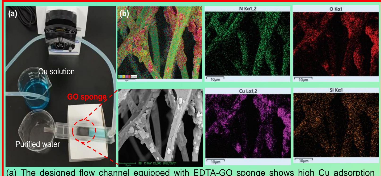
(a) The designed flow channel equipped with EDTA-GO sponge shows high Cu adsorption capacity. (b) The SEM and EDS mapping images of EDTA-GO sponge after Cu adsorption. (c) The picture shows that without siloxane bridge, the EDTA is unable to adhere to the GO surface and releases into the solution.
