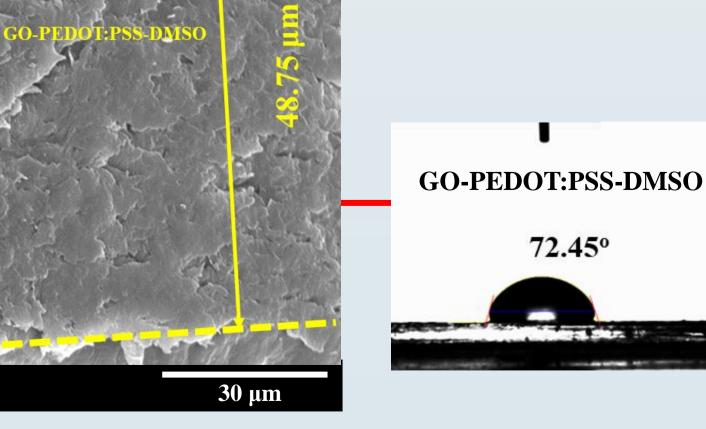
$\succ$  SEM image reveals the interface between P(PEGMA-co-HEMA) and GO-PEDOT:PSS-DMSO layers are good.
