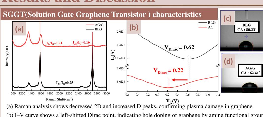
(c)~(d) The reduced contact angle after plasma modification indicates enhanced surface hydrophilicity from amine functionalization.
