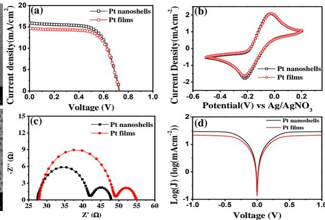
Fig. 3 (a) Photocurrent-voltage(I-V) curves; (b) Cyclic voltammetry; (c) Electrochemical impedance spectra; (d) Tafel curves of the DSSCs with Pt nanoshells and with Pt films.
