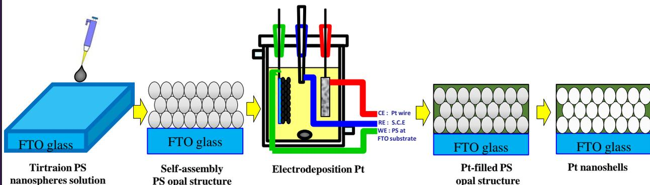
Fig. 1 Schematic diagram of the fabrication of the Pt NSLs. We used the pipette to set the stable capacity the solution of the PS NSs. The solution of the PS NSs self-assembly arrayed in an opal nanostructure. Platinum (Pt) films were deposited onto the PS NSs via the electrochemical deposition method. Toluene can dissolve PS NSs, therefore Pt NSLs will stay.
