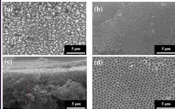
Fig. 2 SEM images of (a) FTO glass; (b) self-assembly polystyrene nanospheres with diameter of 500 nm on FTO glass; (c) electrodeposition platinum on polystyrene nanospheres (side view); (d) platinum nanoshells after polystyrene nanospheres removal.
