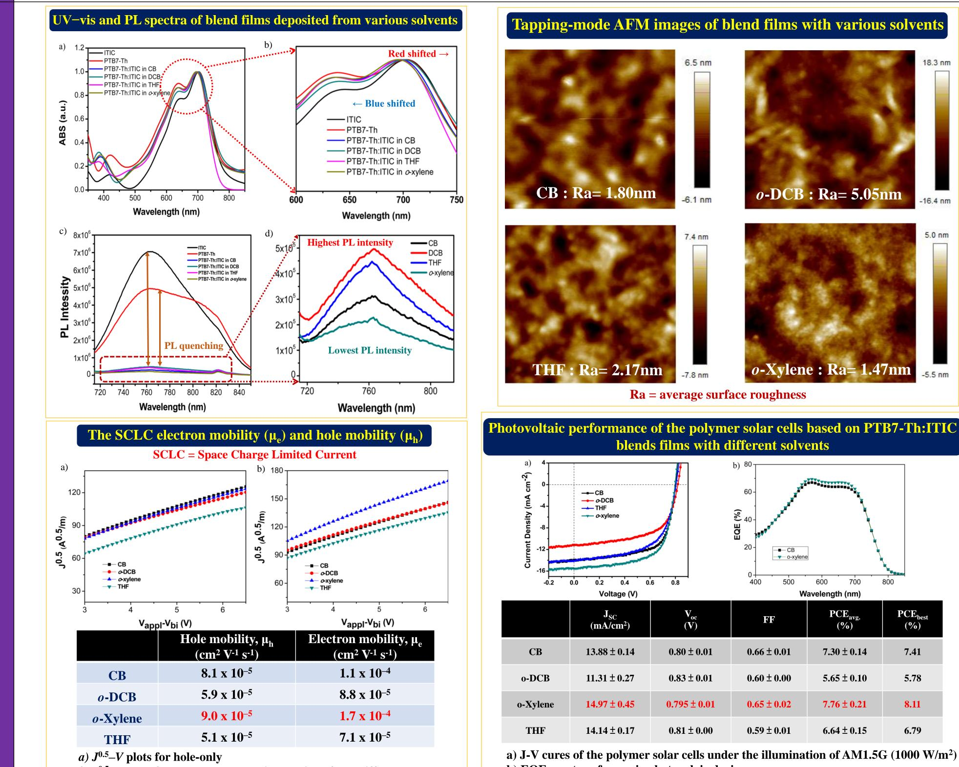
b)  $J^{0.5}-V$  plots for electron-only devices derived from different solvents.
